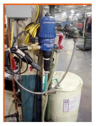
Dosatron dispensers provide on-demand, consistent coolant dilution, compensating for changes in water pressure and flow.
